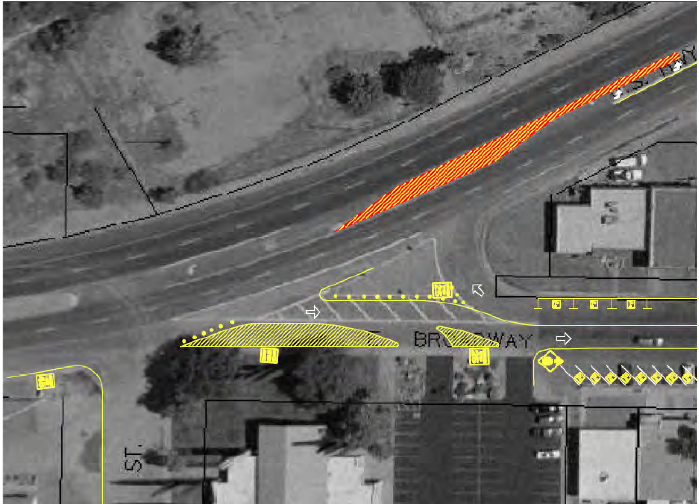
Figure 17: Conceptual Sketch of Suggested Improvements, Including Use of Pavement Markings for a Re-Designed Intersection of US 60/Broadway Street
